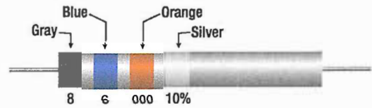
Figure 7-9. Resistor color code example.
