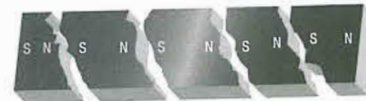
Figure 10-9. Magnetic poles in a broken magnet.
